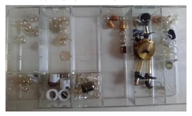
Original HP lamps have the RF coil wound and cemented to the bulb.
