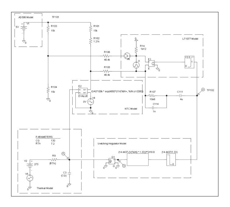
With this model one can easily find answers to several questions: what is the impact of offset bias (< 0.002K), offset voltage (< 0.02K) or resistor tolerance (< 1.4K)?
