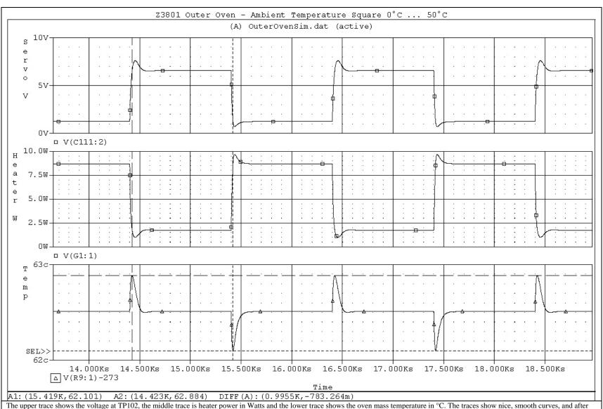
The upper trace shows the voltage at TP102, the middle trace is heater power in Watts and the lower trace shows the oven mass temperature in °C. The traces show nice, smooth curves, and after about 200s the loop has stabilized after a step in ambient temperature
