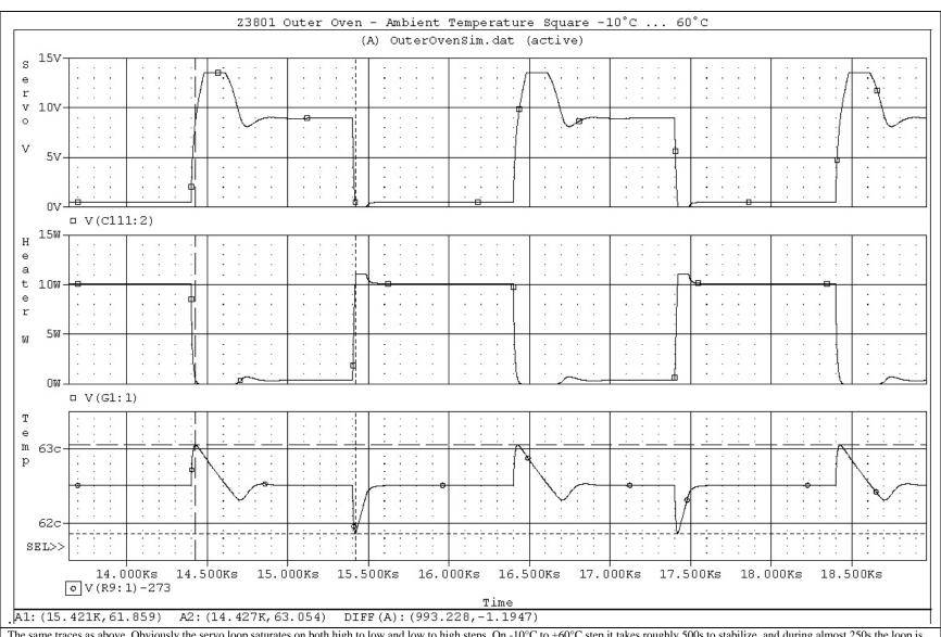
The same traces as above. Obviously the servo loop saturates on both high to low and low to high steps. On  $-10^{\circ}$ C to  $+60^{\circ}$ C step it takes roughly 500s to stabilize, and during almost 250s the loop is unlocked!
