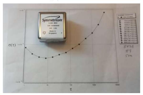
Z3801A or Z3805A Double oven oscillator. This unit was pulled out of my Z3801A as after over many years the aging drifted outside of the DAC range. EFC has been "re-zeroed" to provide years of operation! ADEV 1S-2.01-12, 8S-2.99-12, 64S-3.35-12 \$200.00 free shipping
