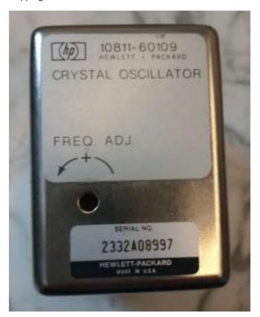
HP 10811A. This unit has the guts out of an HP10811B installed int the case of a -60111 unit. Fully tested and meets A Specs. ADEV 1S-1.01X10-12, 8S-1.56X10-12, 64S-2.57X10-12 \$125.00 free shipping.
